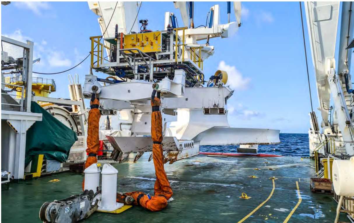
Figure 33: Asso Subsea's Multi-Functional Plough
