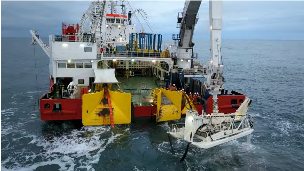
Figure 28: Asso Subsea's Hydroplough during deployment
