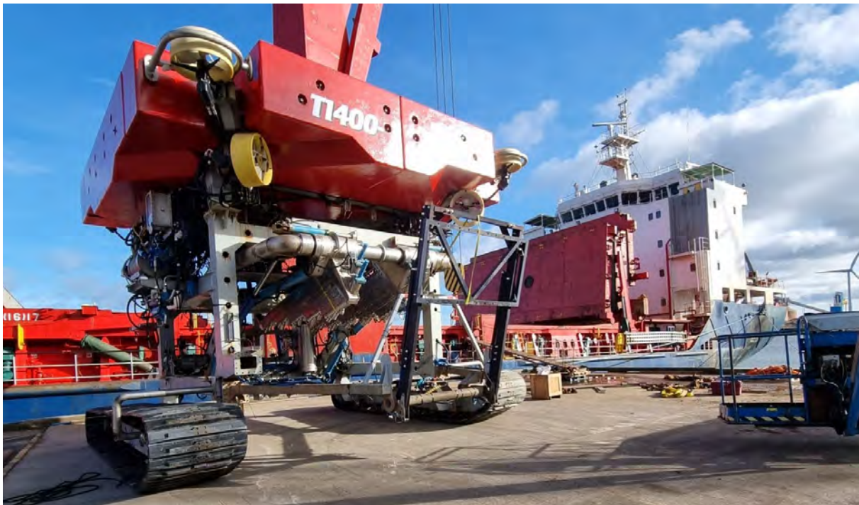
Figure 26: Helix Energy's T1400 Hybrid trenching tool
